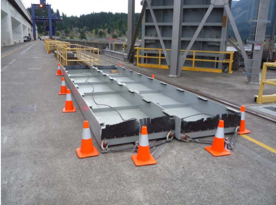
Photo 1-1 TRD slot fillers stored on Bonneville B2 90 Deck
